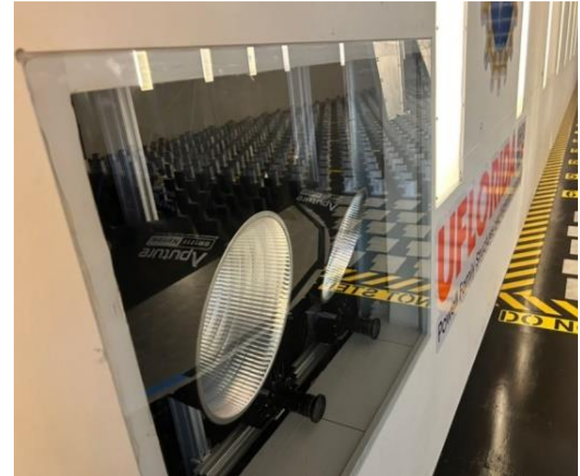
Cameras and lights: Two cameras capture 100 frames per second under flicker-free lights
