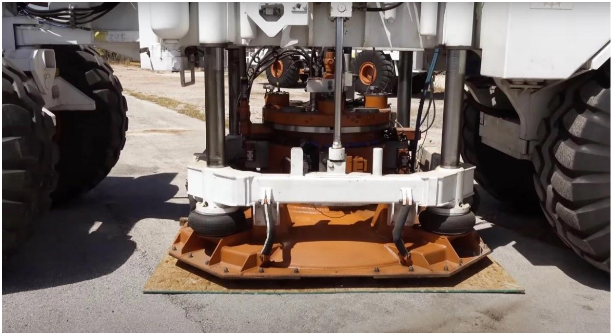
Image 5. Shaking Tool from a Large-Scale Mobile Shaker (Taken from Putzer, 2022)
