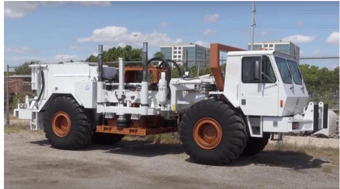
Image 4. Large-Scale Mobile Shaker (Taken from Putzer, 2022)
